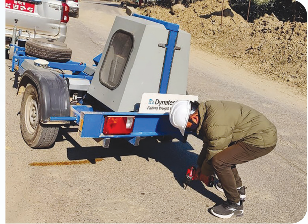
Team from DoR measuring pavement deflection at Dhan Khola to Lamahi section using a FWD.
