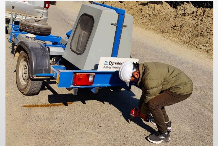
Deflection measurement using FWD
