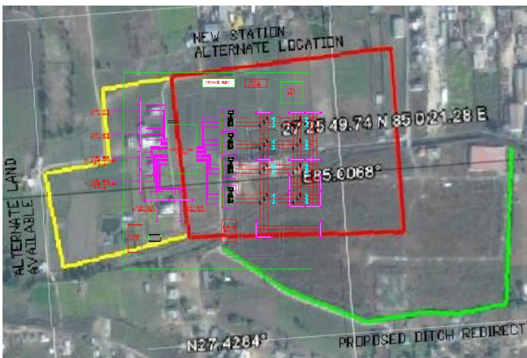
Figure 9. Recommended Location for New Hetauda Substation
