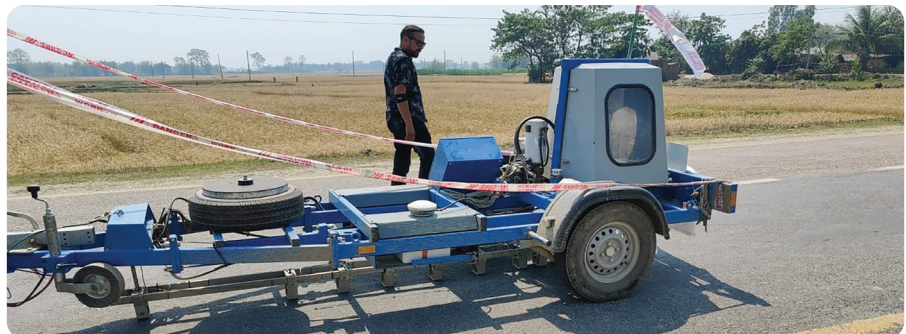
The deflection of road pavement at Nadaha in Saptari district being measured using FWD equipment on 29 March 2023.
