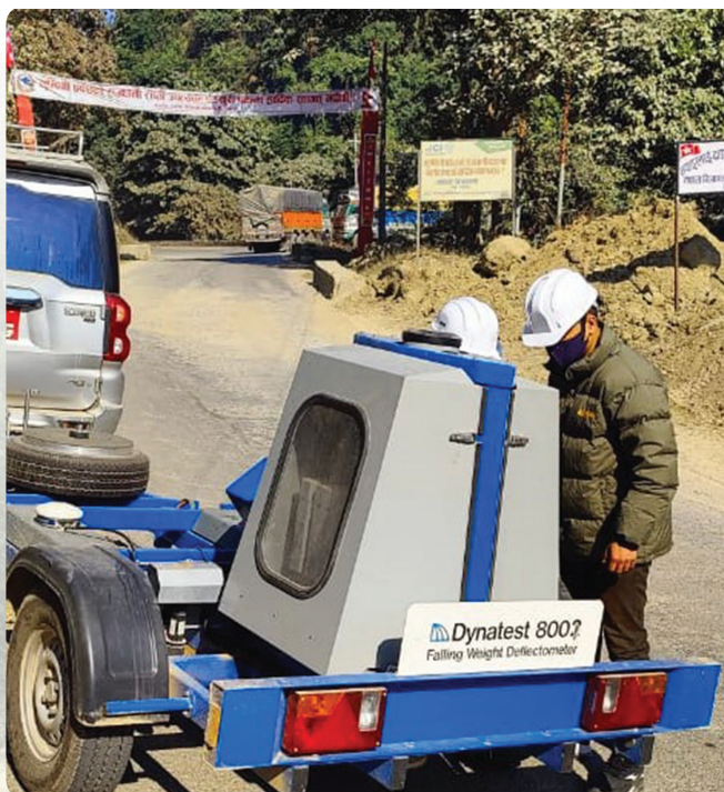
A team from the Department of Roads measuring pavement deflection at Dhan Khola to Lamahi section of East-West Highway.
