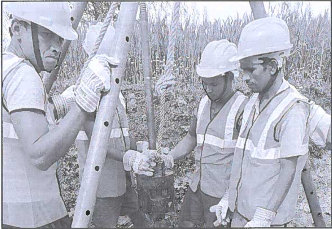
Photograph: Preparatory setup for the SPT test at B1 Hole
