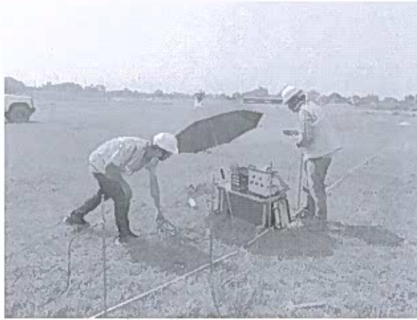
Preparation of profile for soil resistivity test at B7B
