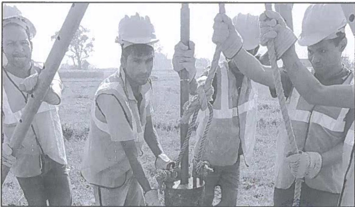
Photograph: Preparatory setup for the SPT test at B7 Hole
