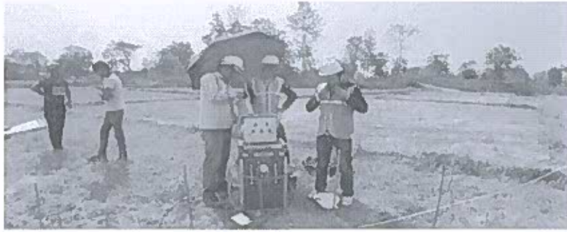
Preparation of profile for soil resistivity test at B2
