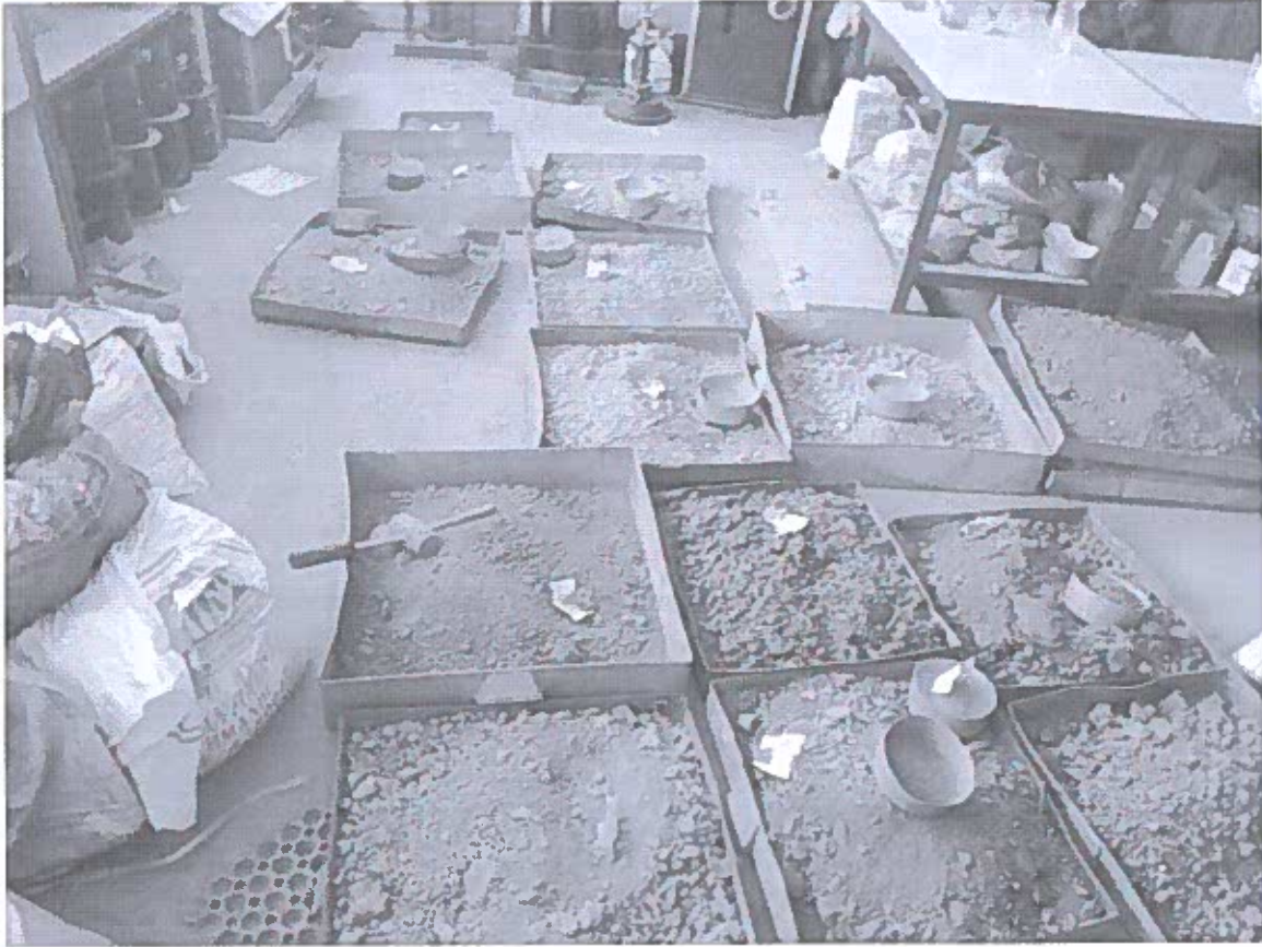
Photograph: Sample separation after Oven dry at ICGS Lab
