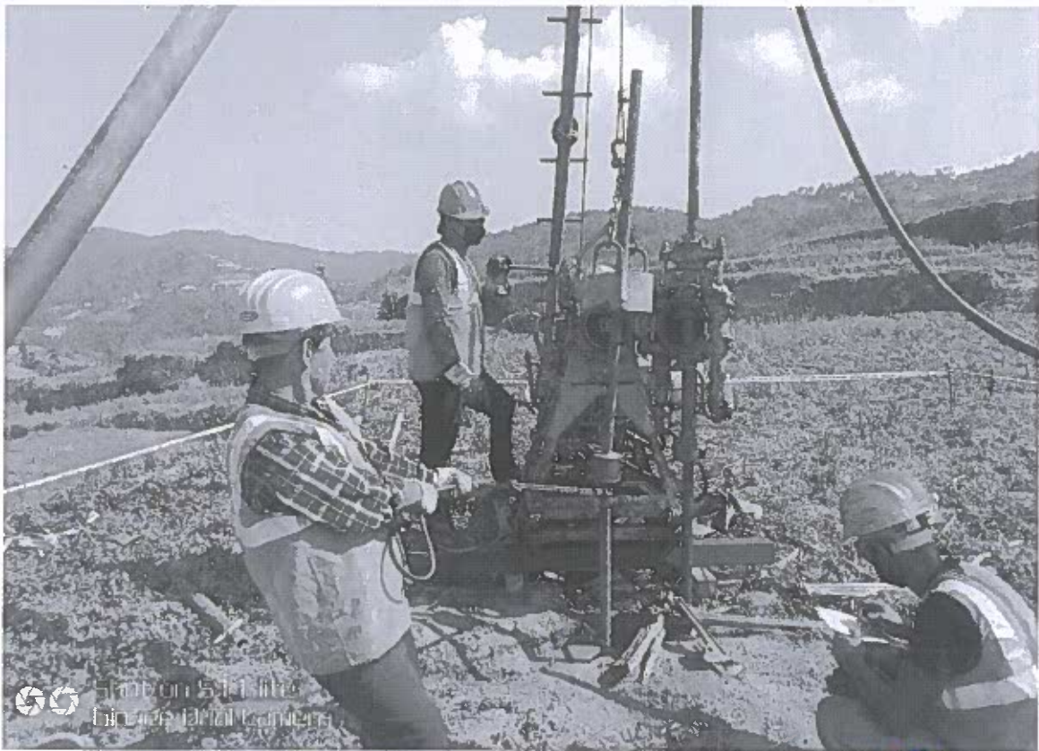
Photograph: Drillers performing SPT test at B49
