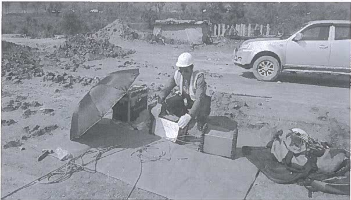
Photograph: Image showing the field setup of the ERT equipment at Ratemate area
