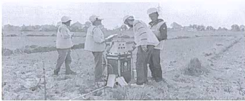
Preparation of profile for soil resistivity test at B6
