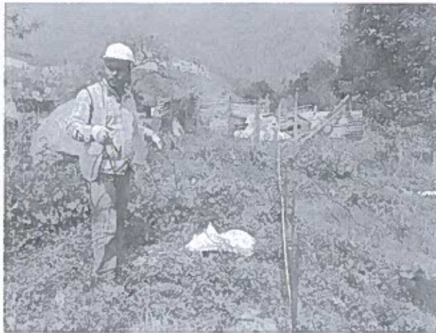
Preparation of profile for soil resistivity test at B52
