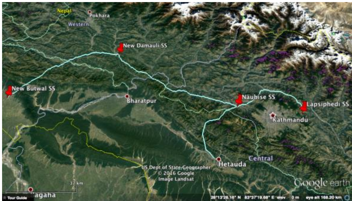
Figure 31 Alignment and Substations of NR1
